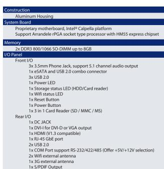
1 x 2.5" SATA HDD or SSD Power Adapter Input: 100-240 VAC, 50-60 Hz Output: 12V/5.4A 65W 2 x half size mini PCle slot (Optional for 3G/WiFi+Bluetooth module) 1x SIM card slot (for 3G appliance) support user accessible **Fanless** Temperature / Humidity Operating: 0°C to 40°C, 0%-90%, non-condensing Storage: -20°C to 80°C, 0%-90%, non-condensing 260 x 153.3 x 57.8 mm (WxDxH) **TBD** ounting Desktop, VESA-mount Certifications CE/FCC Class A
